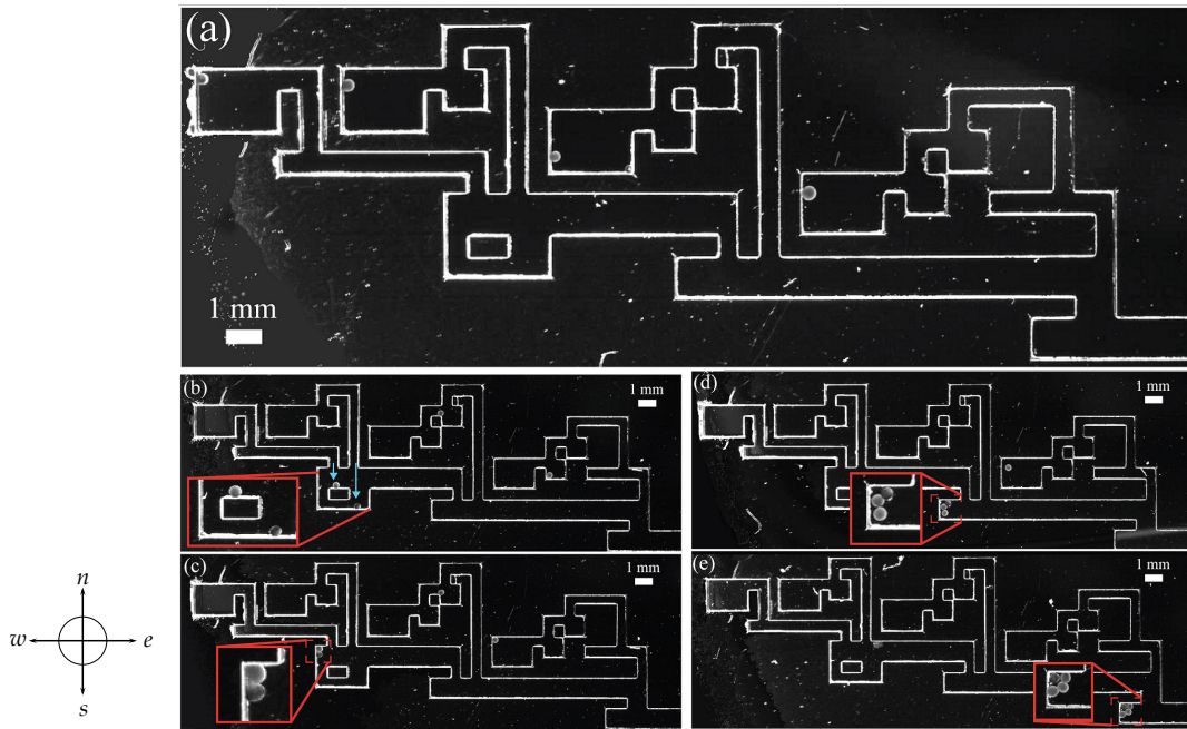
Figure 8.1: A practical demonstration of Tilt Assembly based on alginate (i.e., a gel made by combining a powder derived from seaweed with water) particles on a silicon wafer with obstacles etched in photoresist [202]. The obstacles appear as white lines and block the motion of particles. (a) Alginate particles in initial positions. (b) After control moves of \langle e, s, w, n, e, s \rangle (for east, south, west, north), the alginate microrobots move to the shown positions. (c) After \langle w, n \rangle inputs, the system produces the first multi-microrobot polyomino. (d) The next three microrobot polyominoes are produced after applying multiple \langle e, s, w, n \rangle cycles. (e) After the alginate microrobots have moved through the microfluidic factory layout, the final 4-particle polyomino is generated. This figure originates from [202].
